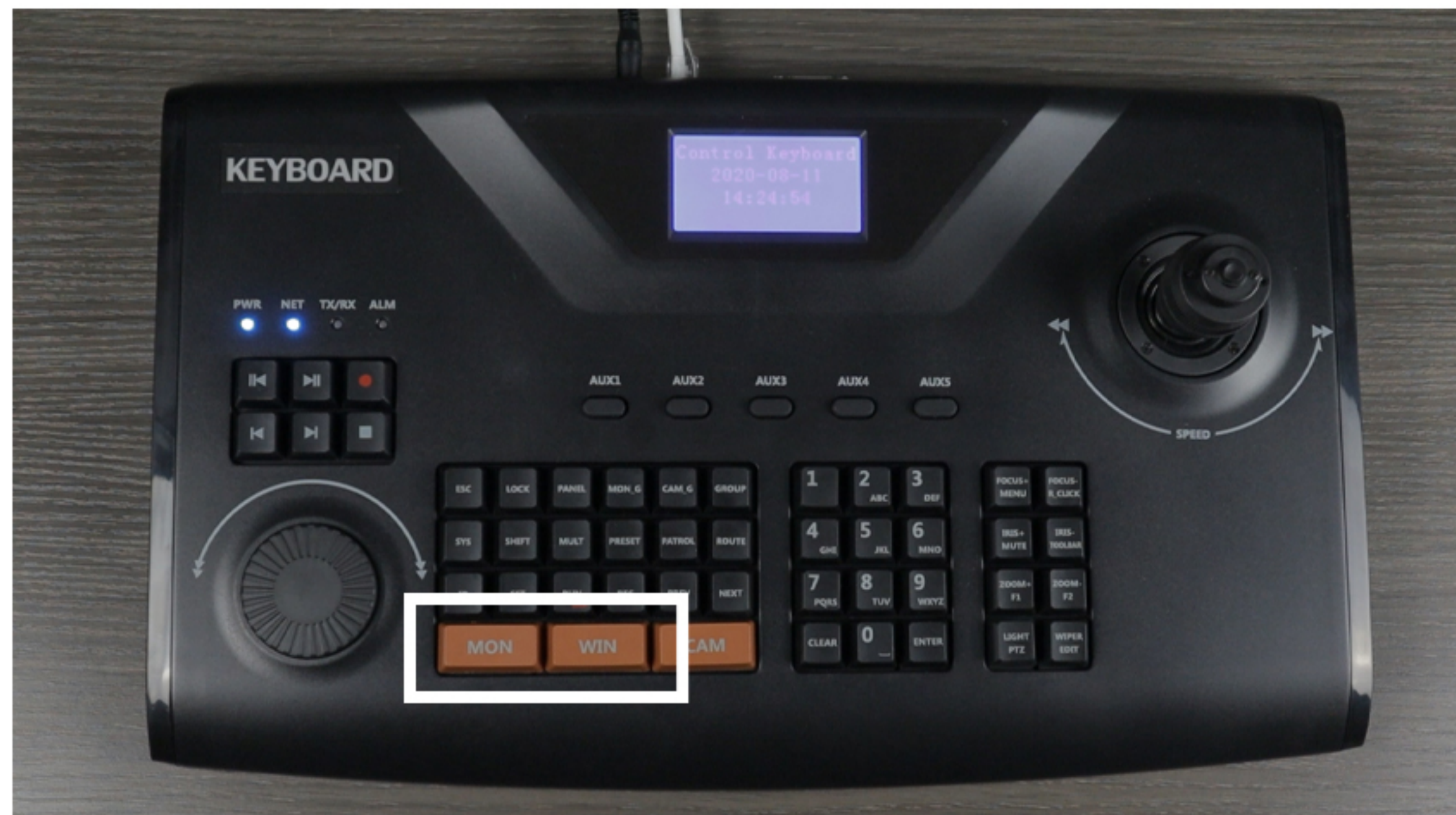
Use the "MON" and "WIN" keys to select a monitor and window respectively.
