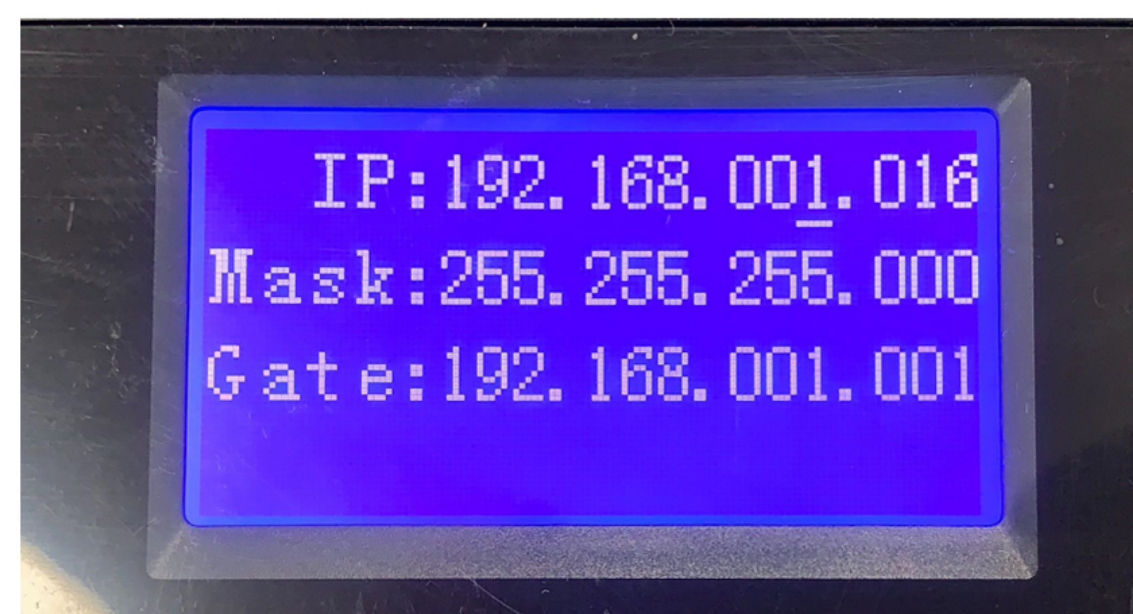
We changed the Keyboard's IP address to reflect the same first three numbers: 192.168.1
