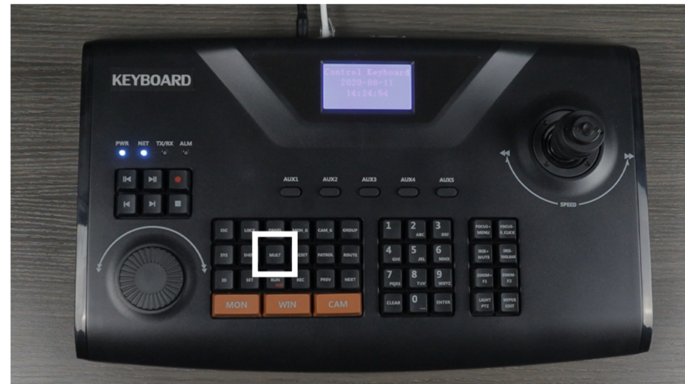
Use the "MULT" key to toggle between multi and single channel views.
