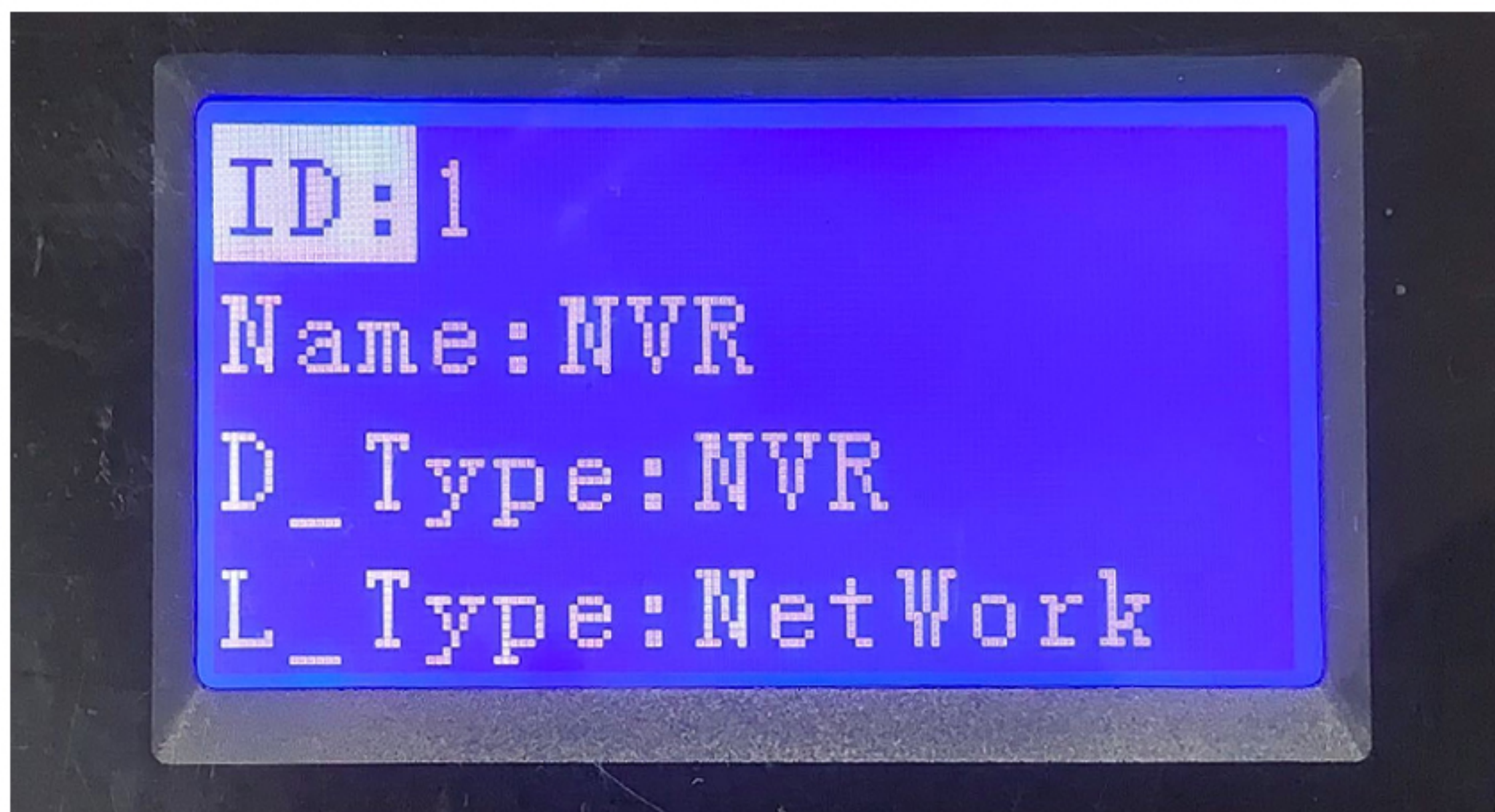
After you type your device ID and press "Enter," your NVR's information will display on the screen.
